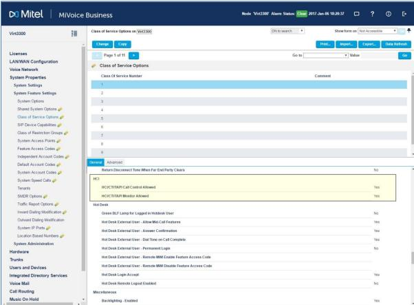
Click the class of service number that is assigned to phones that must be recorded and verify the following two parameters are set as show below:
