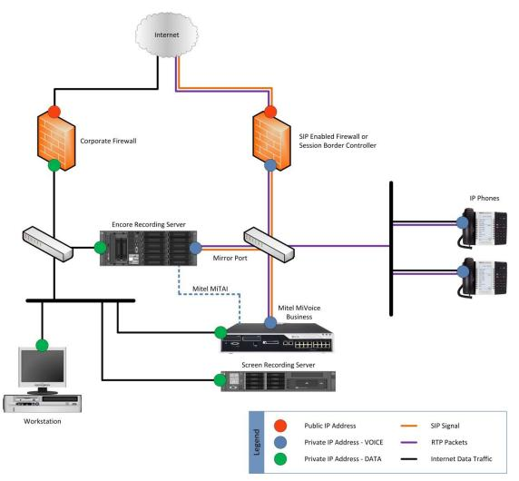
NOTE When recording SIP trunks, DVSAnalytics prefers that all SIP trunk traffic goes through a Session Border Controller (SBC), such as a Cisco CUBE, Ingate SIParator, etc. The SBC's LAN-side port must terminate to a network switch that can provide a SPAN/mirror port to the Encore server.
